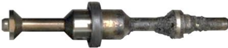
Non-water cooled 3-Way Purge Valve spool after less than 1 year of operation
