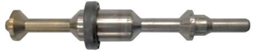
Water cooled 3-Way Purge Valve spool after 3 years of operation with an optimized system
