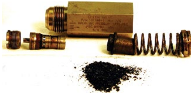
1. Standard liquid-fuel check valve failed to transfer from gas to oil because its operation was prevented by the buildup of coke (pile below valve), removed during disassembly
