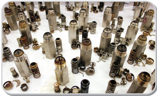
Refurbish existing valves to like-new condition
