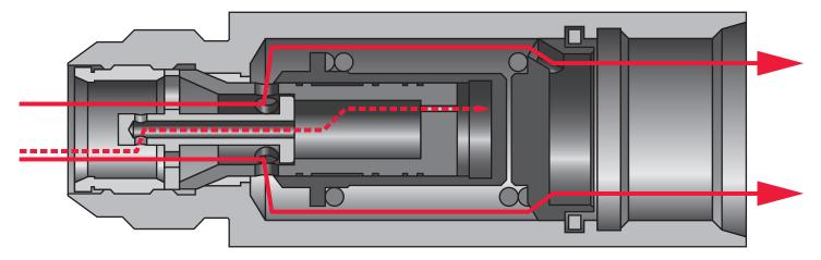
Liquid fuel check valve operation in dual fuel gas turbine applications is extremely severe. The impact of both system and environmental related anomalies on liquid fuel check valves lead to both premature failures of the valve and other fuel system components.
