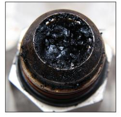
As it relates to gas turbine operation, fuel system integrity suffers greatly from the partial or complete evacuation of liquid fuel when leakage exceeds an ANSI Class 6 standard. Symptoms of check valve leakage related failure include but are not limited to: multiple attempts required to achieve turbine ignition on liquid fuel, high exhaust temperature spreads both at start-up or when transferring from turbine operation on gaseous to liquid fuel.
