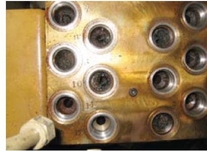
I. Selector Valve required work to unplug ports
