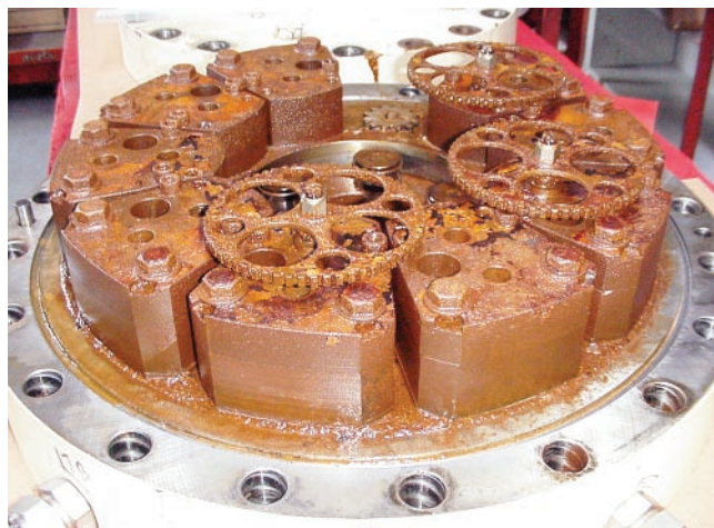
2. Flow divider made of traditional cast iron is susceptible to corrosion that can hamper or prevent operation (left). Upgraded materials are in unit at right
