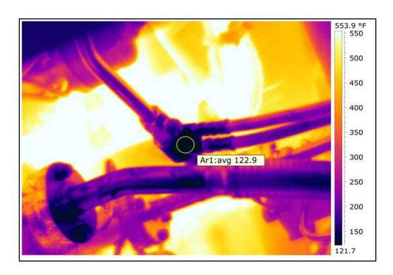
The blue color in the thermal images represents a 122.9 °F cooled valve. All transfers from gas to liquid fuel have been successful, 100% of the starts on liquid fuel have succeeded, and an excess of 30,000 hours of check valve operation have been logged without failure.
