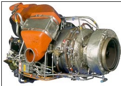
Hamilton-Sundstrand's APS-3200 Auxiliary Power Unit. JASC supplies a variety of fluid and electro-hydraulic control components for the APS-3200. The APS-3200 is mounted on the Airbus A-320 commercial airliner.
