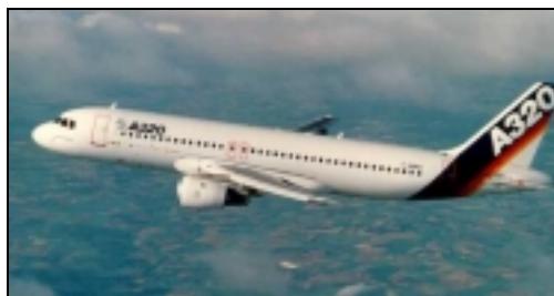
The Airbus A-320 commercial airliner. The Hamilton-Sundstrand APS-3200 APU is used to supply electrical power and air conditioning while the aircraft is on the ground.
