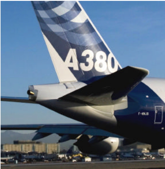
Pictured during the A380's visit to LAX in November of 2007, the tail section houses the PW-980 APU which provides power for the plane's air conditioning, hydraulic systems and electronic systems when the plane's main engines are not running.
