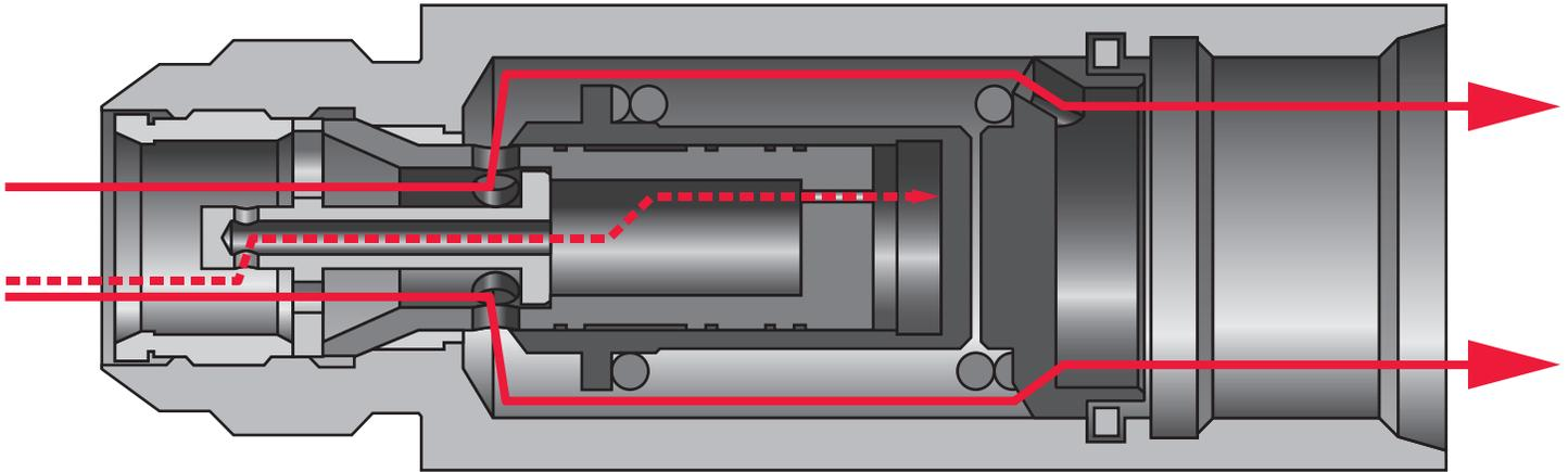
Liquid fuel check valve operation in dual fuel gas turbine applications is extremely severe. The impact of both system and environmental related anomalies on liquid fuel check valves lead to both premature failures of the valve and other fuel system components.
