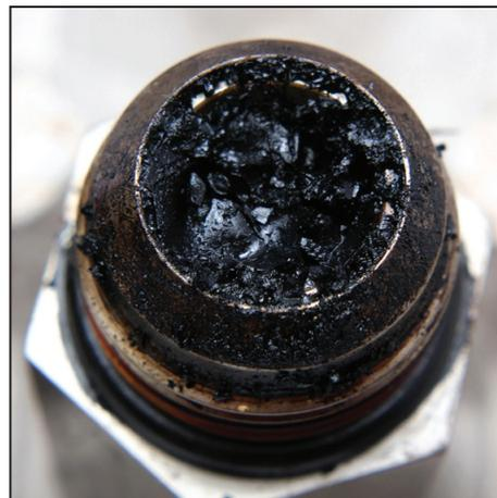
As it relates to gas turbine operation, fuel system integrity suffers greatly from the partial or complete evacuation of liquid fuel when leakage exceeds an ANSI Class 6 standard. Symptoms of check valve leakage related failure include but are not limited to: multiple attempts required to achieve turbine ignition on liquid fuel, high exhaust temperature spreads both at start-up or when transferring from turbine operation
