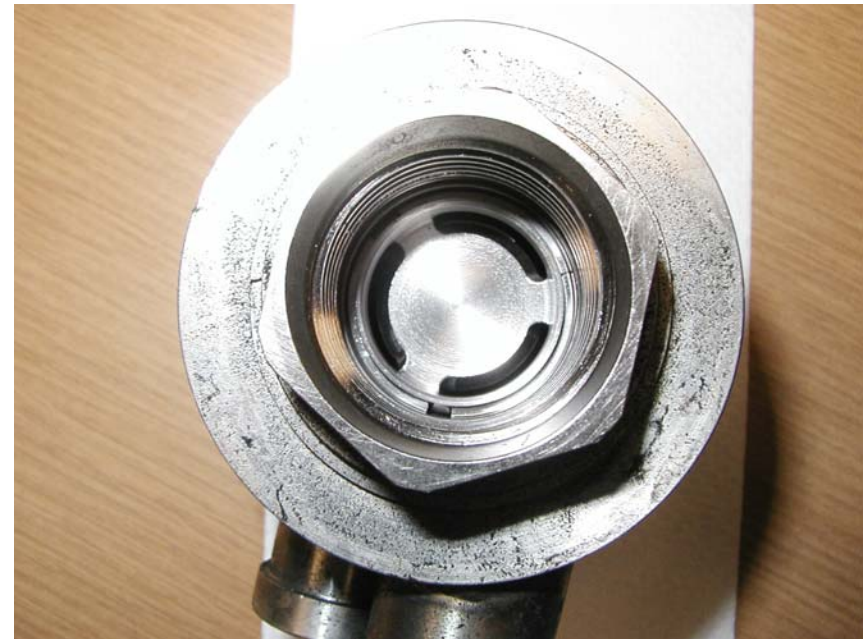
Water Cooled Check Valve
